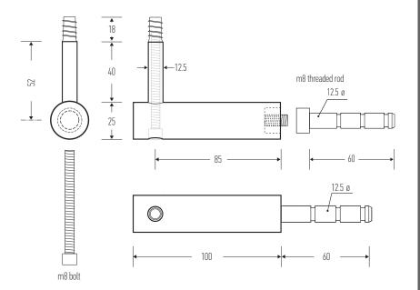
Halliday + Baillie brackets are tested in accordance with both the AS/NZS 1170.1:2002 (Structural Design Actions) standards and the International Building Code, IBC (2003) to comply with the 200lb fall rating.
