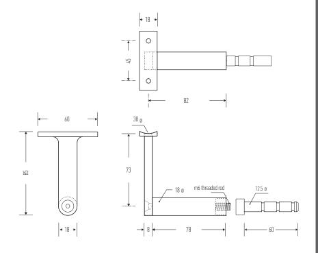
Halliday + Baillie brackets are tested in accordance with both the AS/NZS 1170.1:2002 (Structural Design Actions) standards and the International Building Code, IBC (2003) to comply with the 200lb fall rating.
