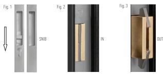
Once you have drawn your slider to its closed position in the frame, simply slide the snib up and the lock bolt and teeth will engage in the receiving strike. When using your key this will lock the snib in place. Please note the key cylinder does not drive the lock bolt itself but locks the snib in place acting similar to a dead bolt function. THE LATCH SHOULD NEVER BE LEFT OUT WHEN PULLING YOUR SLIDER INTO THE CLOSING POSITION. DOING SO RISKS DAMAGE TO THE STRIKE PLATE AND THE LOCK.
