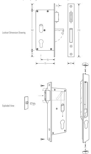
When installed with the snib slid down as far as possible (Fig. 1) the lock bolt and teeth will be retracted inside the body (as in Fig. 2). If the door is slid closed whilst the lock bolt is in the out/locked position (Fig. 3) you risk breakages to both the lock and the strike plate.
