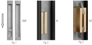
Once you have drawn your slider to its closed position in the frame, simply slide the snib up and the lock bolt and teeth will engage in the receiving strike. The integrated pop out button is activated by pushing to extended and retract and is used to pull the door out of the cavity pocket. THE LATCH SHOULD NEVER BE LEFT OUT WHEN PULLING YOUR SLIDER INTO THE CLOSING POSITION. DOING SO RISKS DAMAGE TO THE STRIKE PLATE AND THE LOCK.
