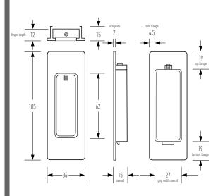
To be used with the HB 604 Timber Fixing Kit on timber doors, sold seperately.
