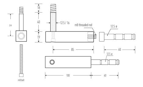
Halliday + Baillie brackets are tested in accordance with both the AS/NZS 1170.1:2002 (Structural Design Actions) standards and the International Building Code, IBC (2003) to comply with the 200lb fall rating.
