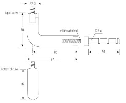
Halliday + Baillie brackets are tested in accordance with both the AS/NZS 1170.1:2002 (Structural Design Actions) standards and the International Building Code, IBC (2003) to comply with the 200lb fall rating.
